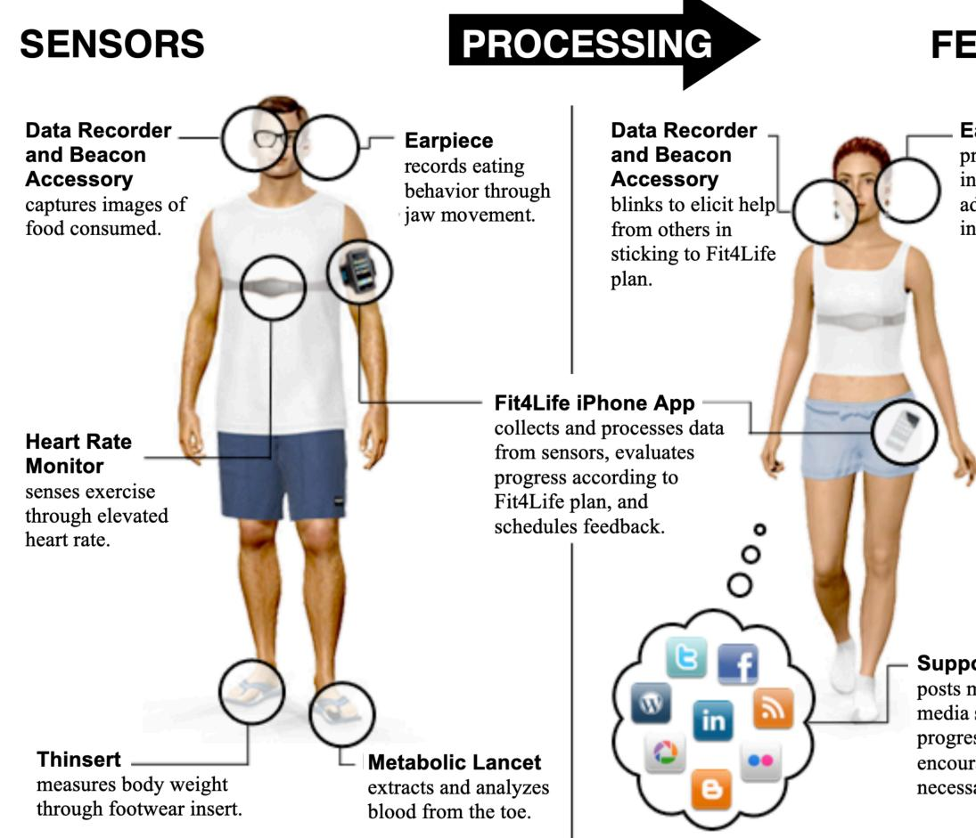
Figure 1. The Fit4Life system in use. All components of the system are shown including sensors, the processing unit, and feedback mechanisms. Certain system components such as The Fit4Life Data Recorder and Beacon Accessory are available in multiple forms (shown here as prescription glasses and fashion earrings) and perform both sensing and feedback functionality.
