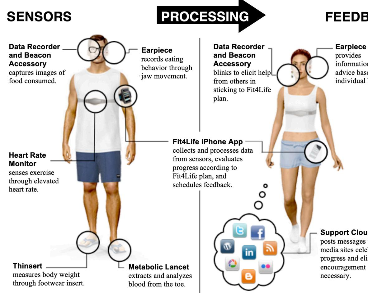
Figure 1. The Fit4Life system in use. All components of the system are shown including sensors, the processing unit, and feedback mechanisms. Certain system components such as The Fit4Life Data Recorder and Beacon Accessory are available in multiple forms (shown here as prescription glasses and fashion earrings) and perform both sensing and feedback functionality.
